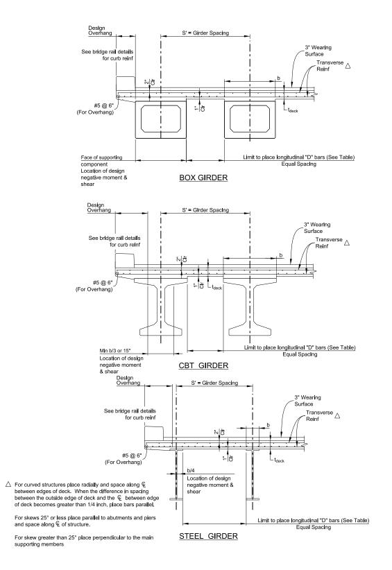
Figure 9-1: Deck Design Table Detail
