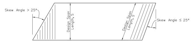
Figure 9-3: Skewed Deck Reinforcing Placement
